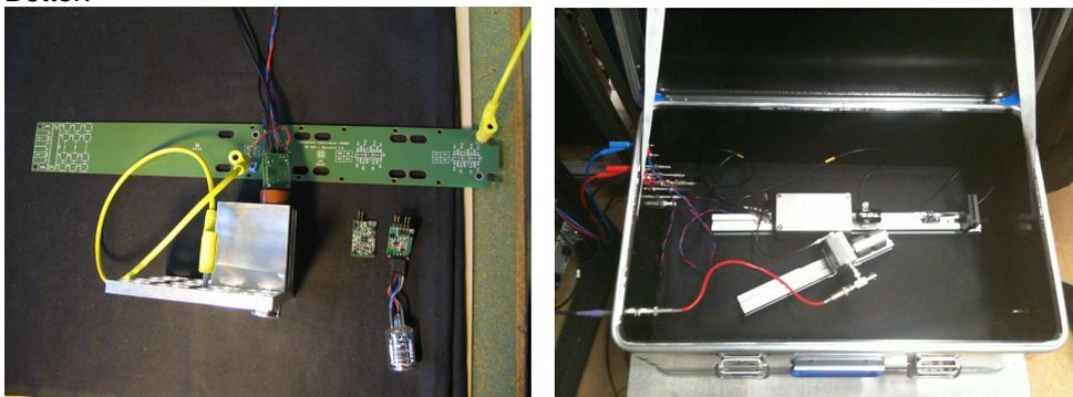
Left: Distribution Board (6 Layer multilayer Board for LV & HV distribution with signal shield and matched 50 Ohm impedance); Right: light tight, shielded Alu-Box with LED & reference PMT
