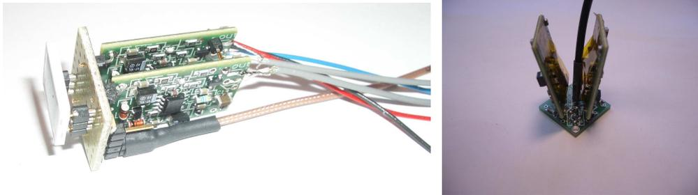
Photo left: two “short” preamps SP883d+prototype DualAPD-PCB 20x20mm +“old” quadratic APD in a socket + cables
