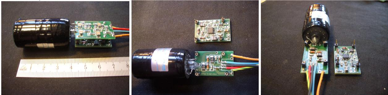
Length of Preamp+R11375MOD Hamamatsu-Tubes: 73mm (with very carefull handling down to 70mm) if distance of PCB's is 8-10mm (the glass exhaust is then overlapped by both Preamp-PCBs).
