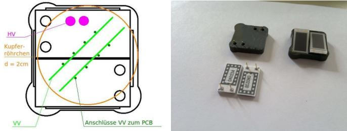
**Note:** The HV is soldered directly to the PCB (placed around the center of the PCB between the preamps). To save cabling, only one HV is available for both APD's . Therefore they must be selected for gain-conformity.
