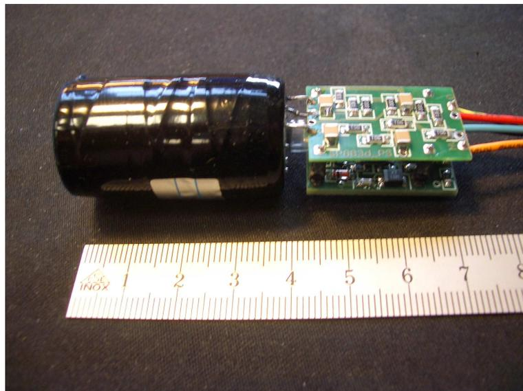
Photo: Preamp SP883d soldered to Hamamatsu VPT
