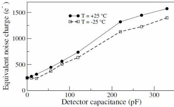
Figure 14: The measured noise performance of the LNP as function of the detector capacitance ( $C_d$ ) at room temperature and at  $-25^\circ\text{C}$ . Measurements are performed by using an ORTEC 450 Research Amplifier with an integration time constant  $T_{int} = 250 \text{ ns}$  and a differentiation time constant  $T_{diff} = 2 \mu\text{s}$ , which corresponds to a peaking-time of  $650 \text{ ns}$ .
