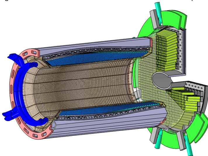
Barrel: 11360 PWO Crystals (11 different shapes), 22720 APDs
