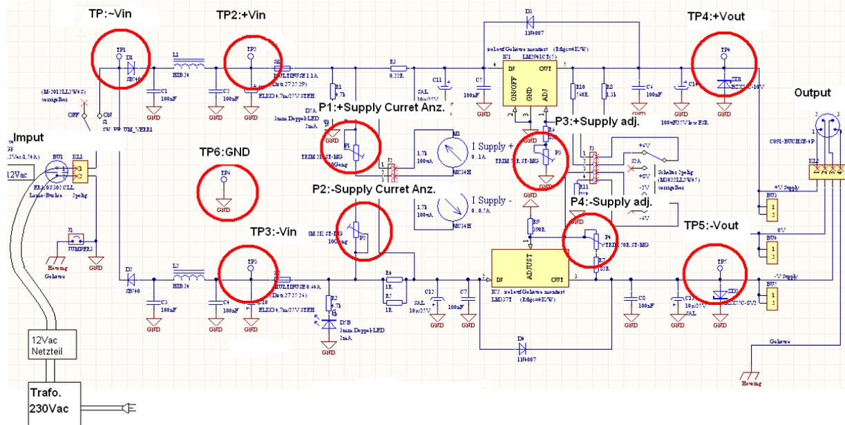
Power Supply type „Basel SP903b“ (shown in photo above) for up to 64 preamps at high rate (here with SP883c and VPT).
