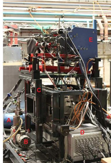
Left: Proto60 with HV; Right: Tests in Mainz; Tank with dry nitrogen gas (A), Vacuum pump (B), X-Y-Support (C), High Voltage Supply (D), Proto60 (E)
