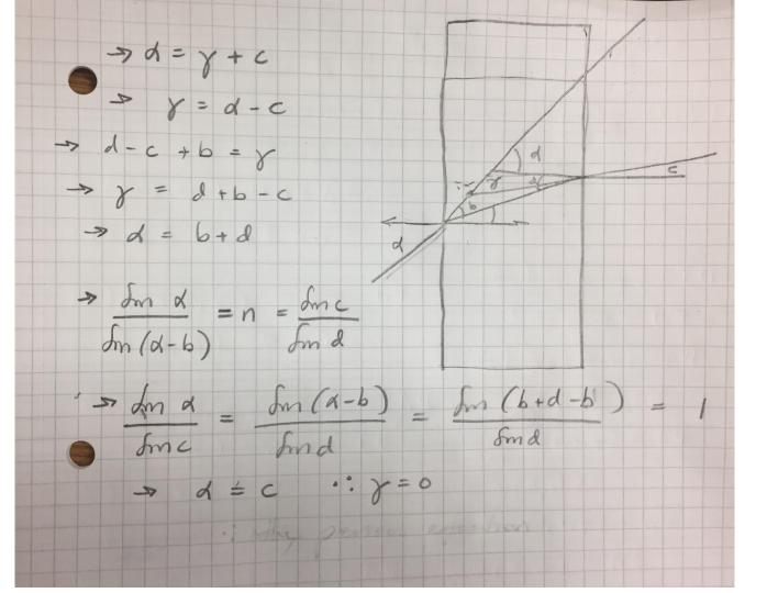
The index cannot be calculated using the first equation when the laser is shone through the body of the prism rather than across the angle
