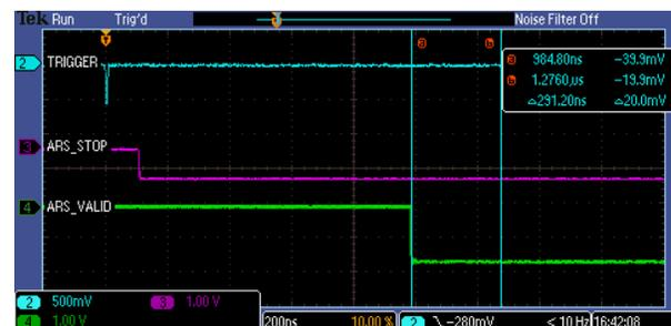
FIG. 11. Timing for an increased gate of 350 ns. The ARS valid and the end of the ARS stop for invalid trigger are pushed later. Their relative timing remains constant ( $\sim$ 290 ns) regardless of the gate width.
