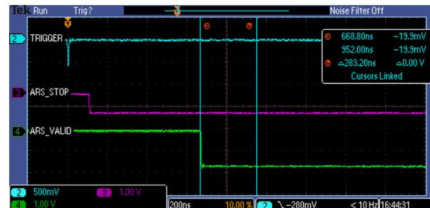
FIG. 10. For invalid triggers the ARS stop ends about 850 ns after it starts, which is about 280 ns after the time when the ARS valid would have been asserted.
