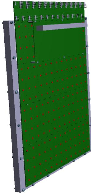
FIG. 2. A panel with 208 LEDs (one in front of each calorimeter block) was used to test the trigger module and its clustering algorithm.
