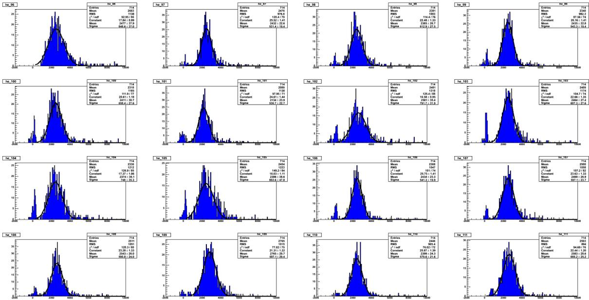
(a) Energy loss by cosmic in each of the 16 blocks of one calorimeter column. A cut on the energy loss in the top and bottom block is applied in order to select vertical events.
