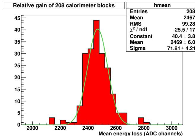
(b) Histogram of the average energy loss in each of the 208 calorimeter blocks after adjusting the gains of each channel. The spread is around 3%.
