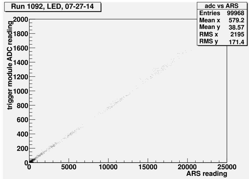
FIG. 5. Trigger module *vs.* the ARS readouts. The correlation between the two sets of electronics shows the correct implementation of a combined DAQ and the synchronization of the events.
