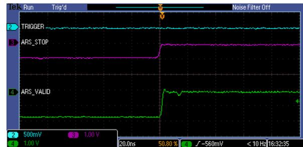
FIG. 9. Signal timing for valid triggers. There is about 560 ns between the ARS stop and the ARS valid for a valid trigger. The ARS stop and valid are true for about 140  $\mu$ s.
