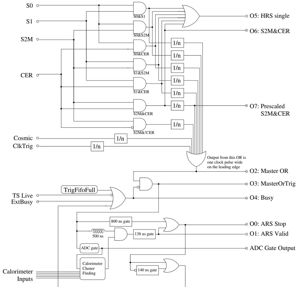
FIG. 3. Diagram of the trigger module internal logic.
