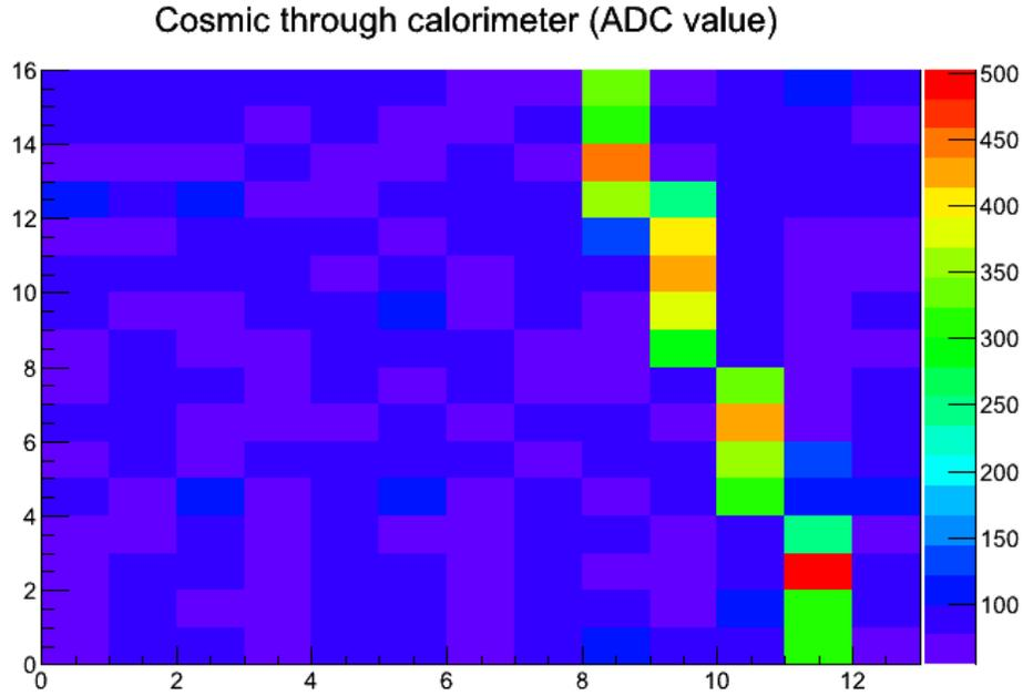
FIG. 7. Cosmic ray travelling through the calorimeter, as seen by the trigger module. The energy scale shows the ADC value recorded by the module.
