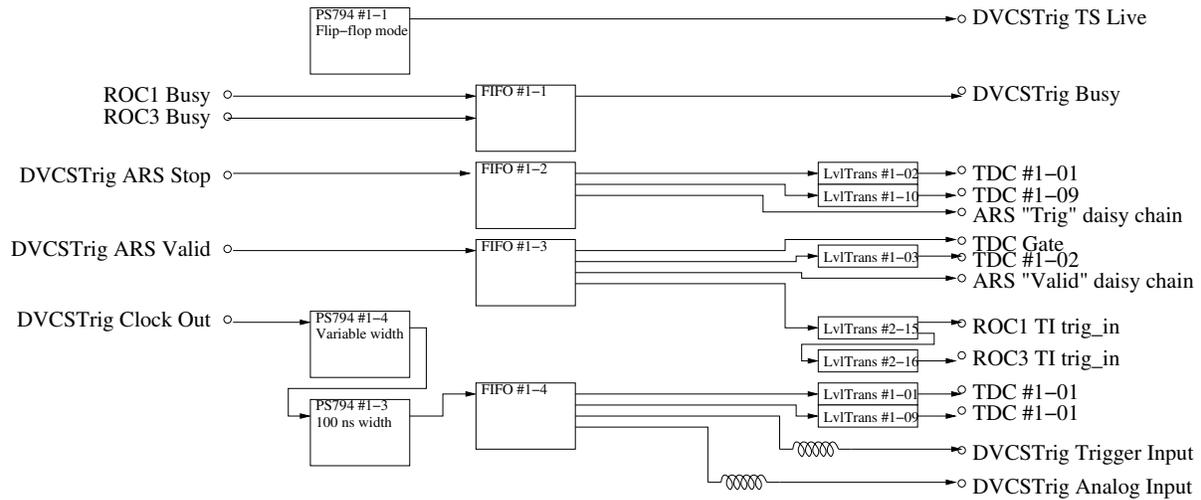
FIG. 4. External logic as used in DVCS test stand.
