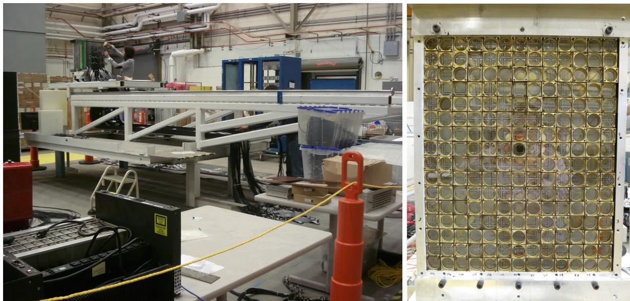
FIG. 1. Left: overview of the DVCS setup in the Test Lab. Right: Front view of the calorimeter, showing the array of 208  $\text{PbF}_2$  blocks.
