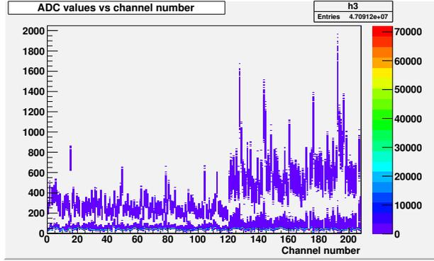
(a) ADC value recorded by the trigger module for a typical LED run, as a function of the calorimeter channel number.
