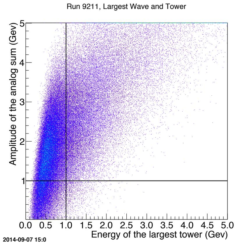
FIG. 12. Analog sum *vs.* largest  $2 \times 2$  cluster, from DIS data taken during the 2010 DVCS run. The analog sum contains too much noise to make it an efficient trigger for the experiment.
