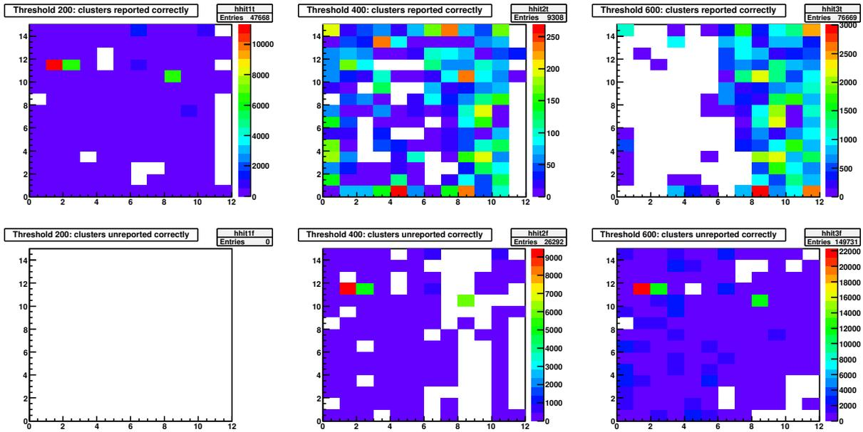
(b) For three different values of the threshold (columns), position of the highest signal cluster when the existence of a cluster was correctly reported (top) and when the absence of a cluster above threshold was correctly reported (bottom). Both cases are successfully tested across the surface of the calorimeter at some value of the threshold. Not a single event was reported incorrectly.
