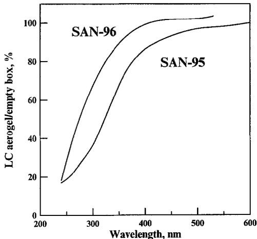
Fig. 1. The relative light collection coefficient for two types of aerogels with  $n = 1.05$ .
