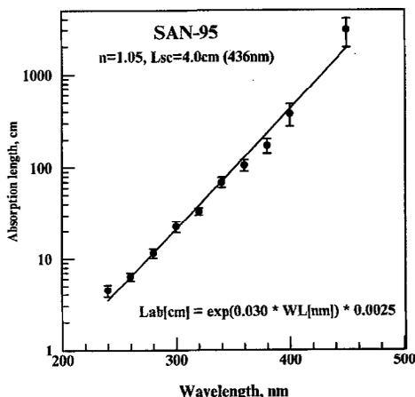
Fig. 2. Absorption length of aerogel as a function of wavelength.
