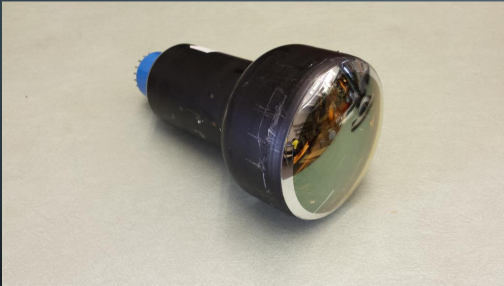
XP4500/B PMT, used in detectors like Cherenkov detector at JLab
