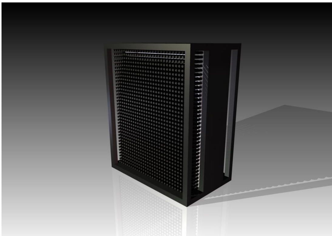
Figure 26: Back face. Each crystal has one PMT attached.
