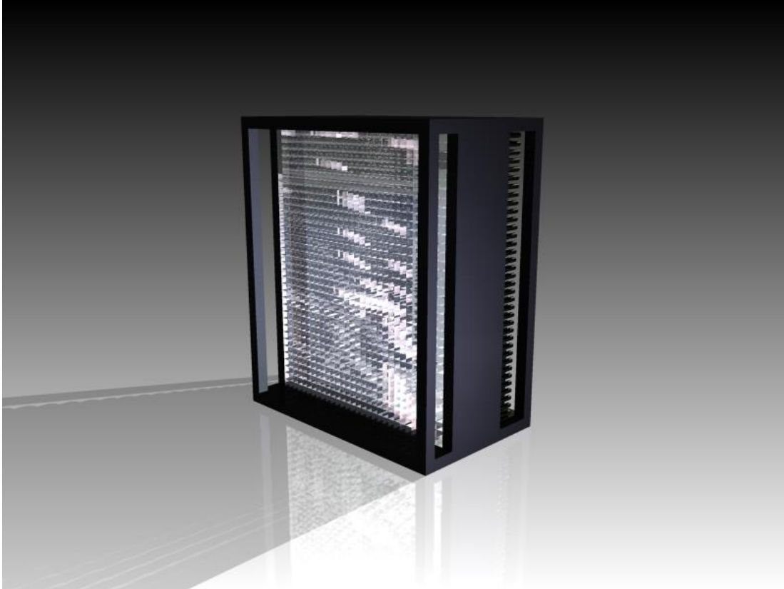
Figure 22: Front face of the Calorimeter with 30 x 36 Lead-Tungsten crystals (PbWO 4 ).
