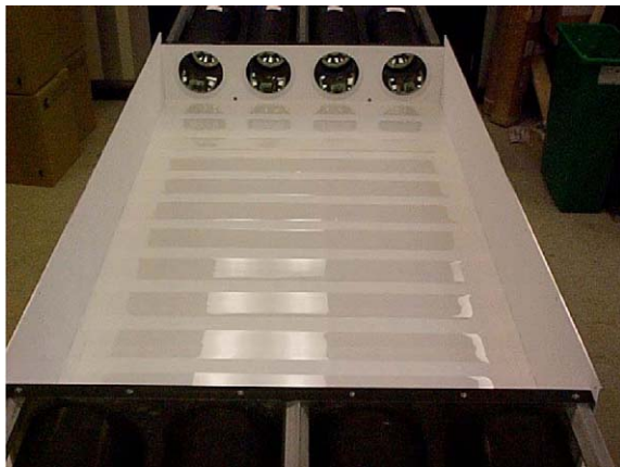
Fig. 3. A complete Cherenkov counter without the back cover, showing the aerogel, reflective surfaces and one end of PMTs.
